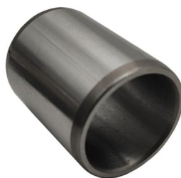
Shaft Sleeve OD=25 mm ID= 20 mm L = 28.5 mm P/N:0472105823 POS:18# For Pump Type: RA0025/0040
